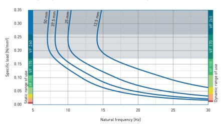
Natural frequency of a single-degree-offreedom system consisting of a fixed mass and an elastic bearing consisting of VIKAFOAM VF 170 on a stiff subgrade.
